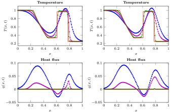
$\Delta t=0.4\Delta x$ ,  $\Delta x=0.01$ ,  $N_v=80$ , K=2 and  $\delta t=\varepsilon$ , for  $\varepsilon=10^{-1}$  (blue dots),  $10^{-2}$  (purple dots), and  $10^{-5}$  (green dots). Red line: hydrodynamic limit  $\varepsilon\to 0$
